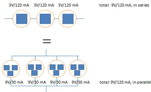
Figure 3: Two manifestations of a 9V/120 mA array using single- and triple-die packages, the second one featuring 4 iso the straightforward 3 LEDs (+33% LEDs).
