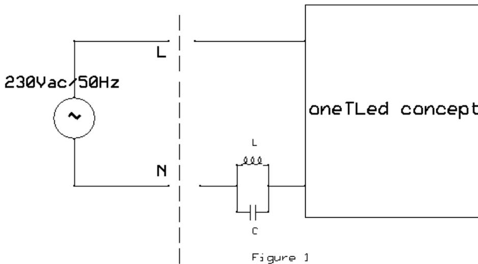
Figure 1: Schematics of AC/Mains Voltage Compatible oneTLed; right from dotted line is the OneTLed lamp.
