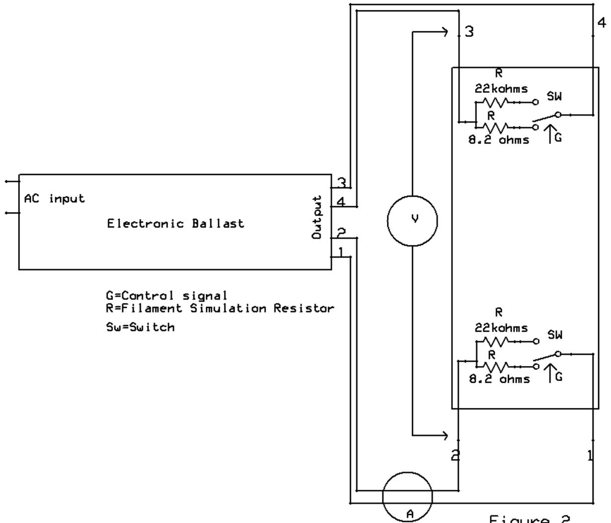
Figure 2: Schematics of filament simulation resistor cut-off technology; after a certain time the switch (30 msec was found to work fine) in series with the filament resistor R opens, and replacement the low resistance of the filament resistors (typically 8 Ohm) by a higher resistance value (advised 22 kilo Ohm).
